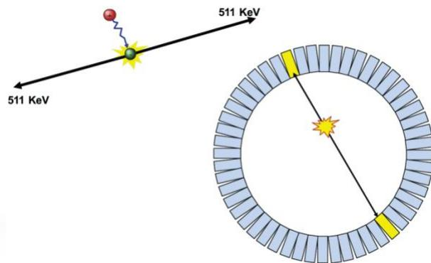
Fig. 2: In PET, two 511 keV gamma photons from a positron electron annihilation have to be detected and correlated.
