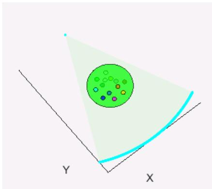
Figure 1. Fan beam CT simulation setup in ImaSim
